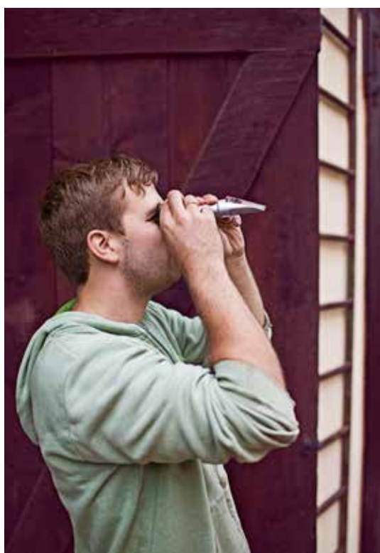
Measuring must weight with a refractometer 20°C (68°F)
